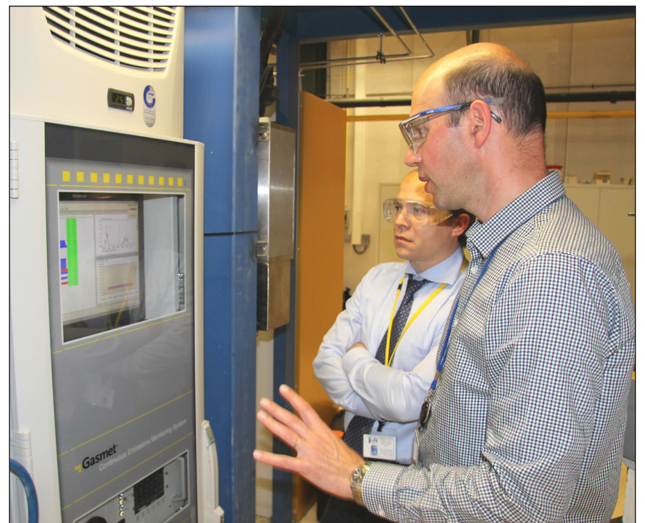
A fixed FTIR analyser provides near real-time monitoring of flue gas treatment efficiency
